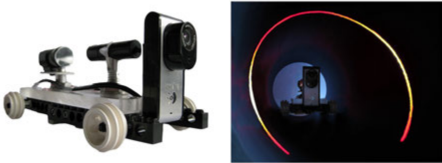
FIGURE 8.12 First prototype ASV system by Drost [28] consisting of frame, mirror, laser and camera
