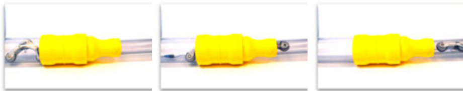
FIGURE 12.16 Robot taking a diameter change from 110 mm to 63 mm
