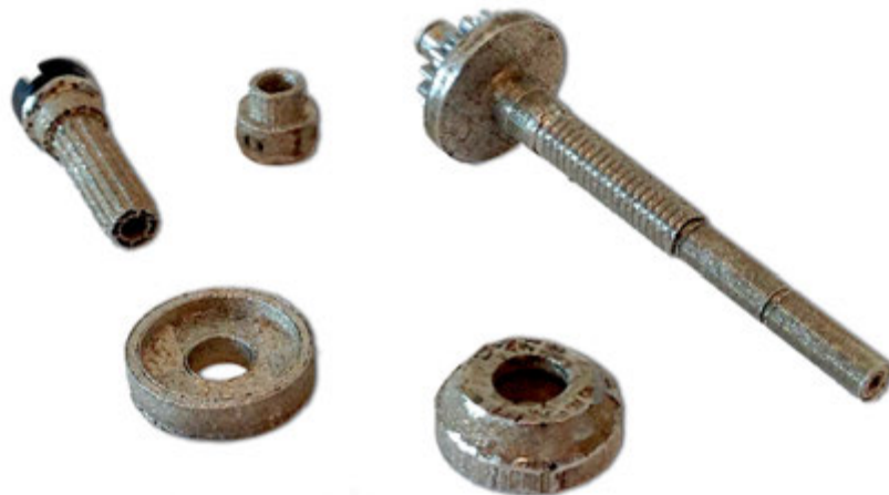
FIGURE 11.8 Finished parts (after some considerable rework using a rotary tool)
