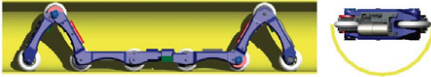
FIGURE 4.4 Top view and side view of robot model in 125 mm pipe - image from [104]
