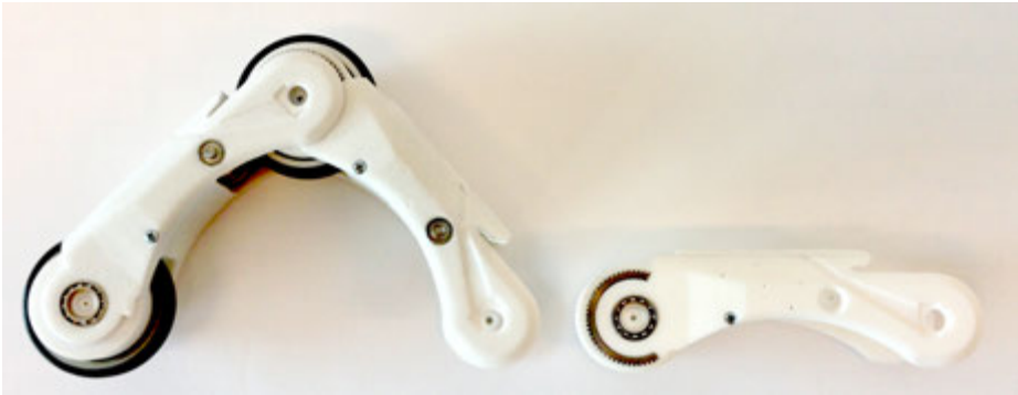
FIGURE 11.11 Three modules printed in PA3200
