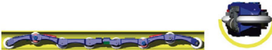
FIGURE 4.5 Top view and side view of robot model in 63 mm pipe- image from [104]
