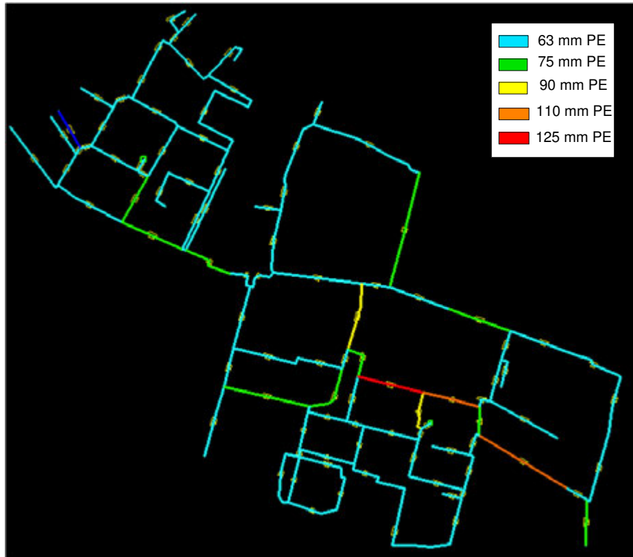
FIGURE 2.4 Schematic image of a part of the gas distribution grid in Arnhem - screenshot from KIWA documentation software
