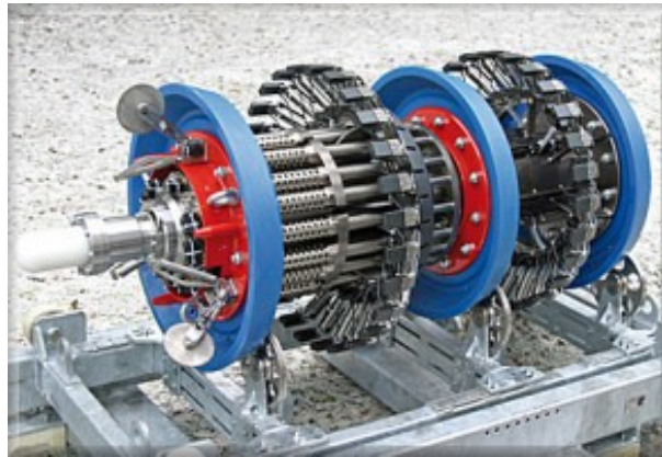
FIGURE 3.5 Geometry (or caliper) PIG by ROSEN- image courtesy of ROSEN Inspection Systems
