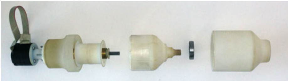
FIGURE 9.3 'exploded' view of the parts used for the spooling system
