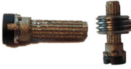
FIGURE 11.9 Drive shaft with fitted oldham coupling plate and worm gear
