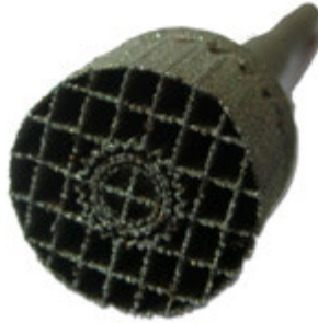
FIGURE 11.5 Shaft with the support material that needs to be removed
